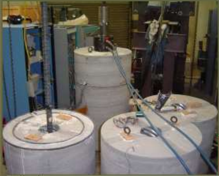
Pull out Test Large Bar – Grouted Duct
