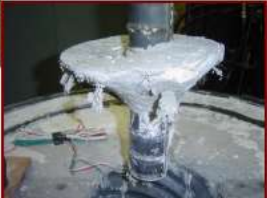
Pull out Test Large Bar – Grouted Duct
